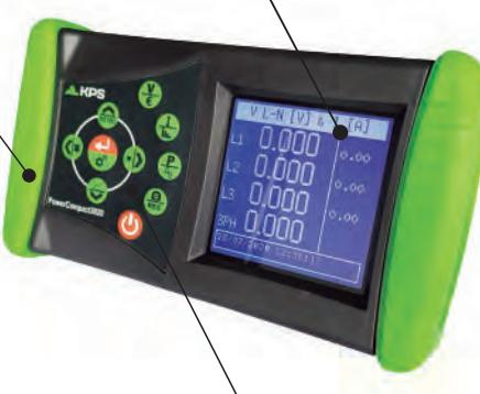
Elegant membrane keypad with 10 buttons with dual function provides an easy and intuitive navigation menu.
